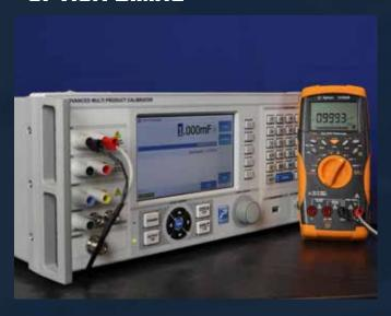
Included in -SYS units, the simulated option provides for resistance calibration between cardinal points and gives a continuous resistance range from 0 Ohms to 1 GOhms, with variable capacitance from 0.95uF through to 100mF.
