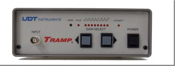
The UDT Instruments TRAMP is a transimpedance amplifier (current-to-voltage) instrument which provides a low input impedance to accurately measure the short circuit current of phototransducers such as silicon and germanium photodetectors, vacuum photodiodes and photomultiplier tubes.
