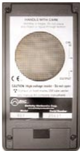
The back panel of the palmRAD 907 shown above features the 2-inch pancake GM detector.
