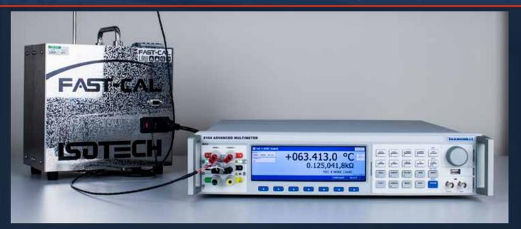
Included standard with the 8104 is the ability to measure temperature through 2, 3 and 4 wire PRT's and SPRT's with inbuilt support for both IEC 751 and ITS 90 probe coefficients. The 8104 displays both the calculated temperature and resistance simultaneously as well as the ability to ratio between two probes
