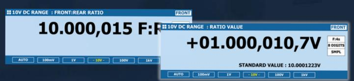
The 8104 comes fitted with electronically switchable rear panel inputs as standard enabling the 8104 to perform ratio measurements between two sources. Combined with exception linearity the ratio functionality can replace the use of Kelvin Varley Dividers in precision voltage measurement.
