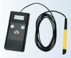
The Trek Model 876 (±2kV) and Model 884 (±20kV) Hand-Held Electrostatic Voltmeters provide accurate, noncontacting measurements of electrostatic surface voltage for ESD applications in either ionized or non-ionized environments.
