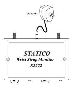
2. Connect the Monitor to the Ground via Grounding Wires
