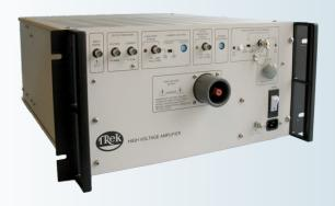
Trek Model P0621P (+) / P0621N (-) is a high-voltage DC-stable piezo driver/amplifier designed to provide precise control of output voltages in ranges that are customer specified within a range of available settings. It is configured as a noninverting amplifier with a variable DC gain. An inverting amplifier configuration is also available.
